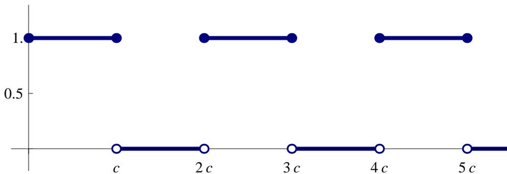
Figure 5: A periodic on-off switch
