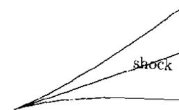
Figure 12.6.11: Envelope of characteristics, locus of intersections of neighboring characteristics.
