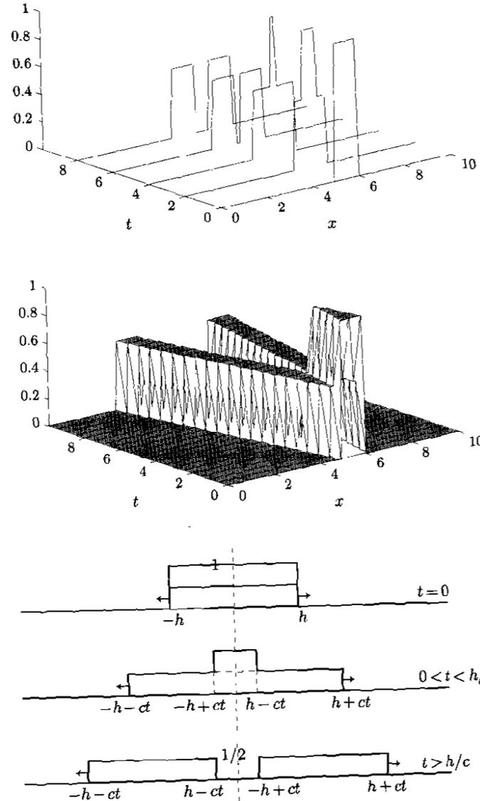
Figure 12.3.2: Initial value problem for the one-dimensional wave equation.
