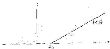
Figure 12.2.1: Characteristics for the first-order wave equation.
