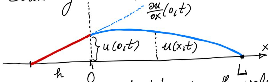
the red super-glued part determines the value of the slope of the string at 0, that is  $\frac{\partial u}{\partial x}(0,t)$ :
